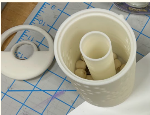
(Fig no.13) 3D-printed scented rattler assembly
