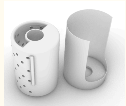
(Fig no. 11) CAD model of scented rattler
