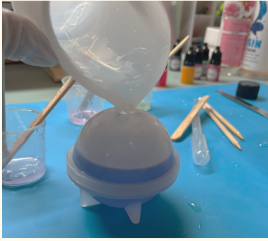
(Fig no.29) Resin shapes being poured into silicon sphere mold
